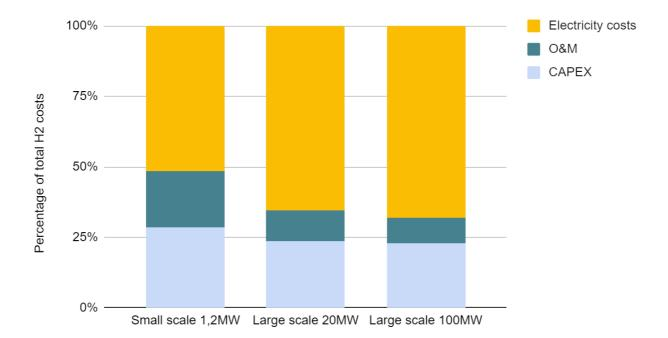
The investment share of CAPEX will be more important than pictured to **include the conditioning and transport of hydrogen to the point of use**; The sizing of the compression unit and storage varies a lot depending on the customers requirements. Additional systems for the conditioning of hydrogen will be necessary to transport the molecules. Depending on the design it could increase by 15% to 30% the total investments.
